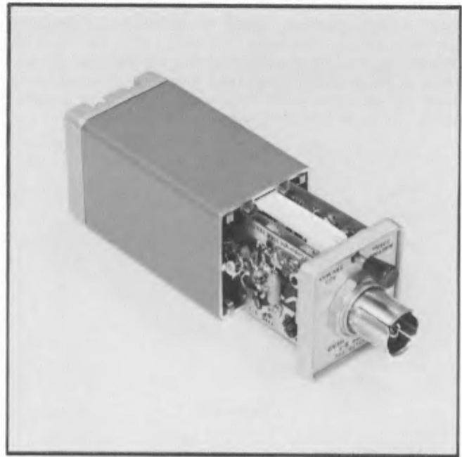
Fig. 5-14. Correct board and latch positions when reinstalling the Sampling Head case.
