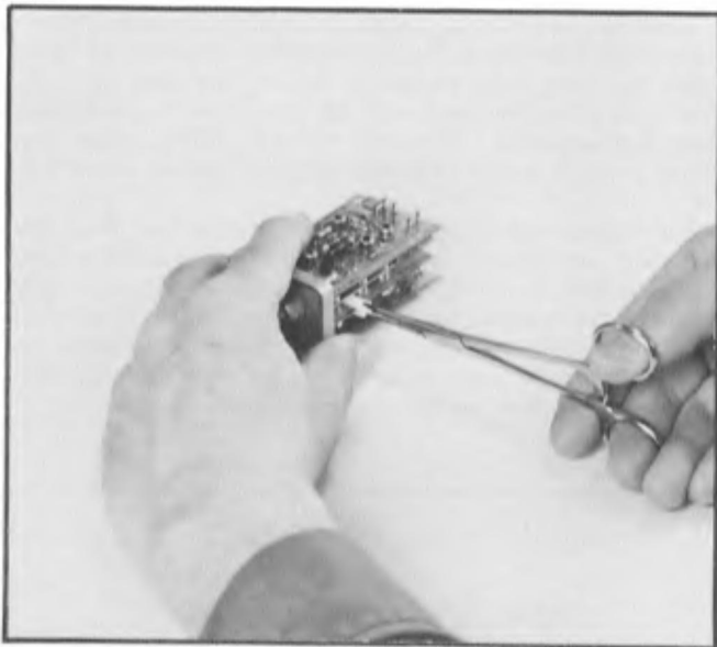
Fig. 4-2. Removal or replacement of sampling bridge diodes.
